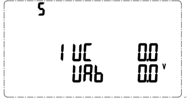
Phase voltage U_c and line voltage U_{ab}
